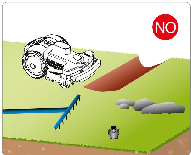
The slope must not increase at least 35cm inside or outside the perimeter wire. If these instructions should not be complied with, while the robot is working on sloping areas and detects the wire, its wheels could slip and make it leave the working area.
