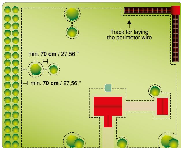
The minimum passage allowed is **70 cm** (27.56") from each edge of the perimeter wire. The perimeter wire must be positioned at a distance of (to be indicated below) from any objects outside the lawn; therefore, the necessary space for passing must be **140 cm** (55.12") if there is a wall or hedge on both sides.
