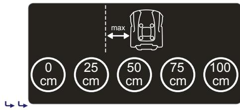
"0 cm". This setting is recommended for complex gardens with many obstacles near the perimeter wire and gardens with narrow passages. The robot will position its wheels on either side of the perimeter wire to return to the charging station.
