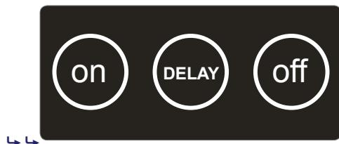
**ON:** when rain is detected, the robot returns to the charging station. At the end of the charging cycle, the robot resumes its normal operation if the sensor no longer detects rain.
