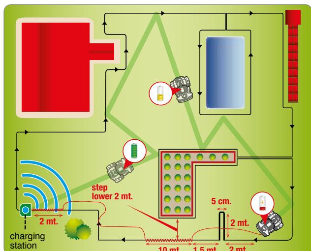
If narrow passages are present or the arrow for quick re-entry to the charging station, the wire must be positioned in a special way, called “Recall on the wire.”
