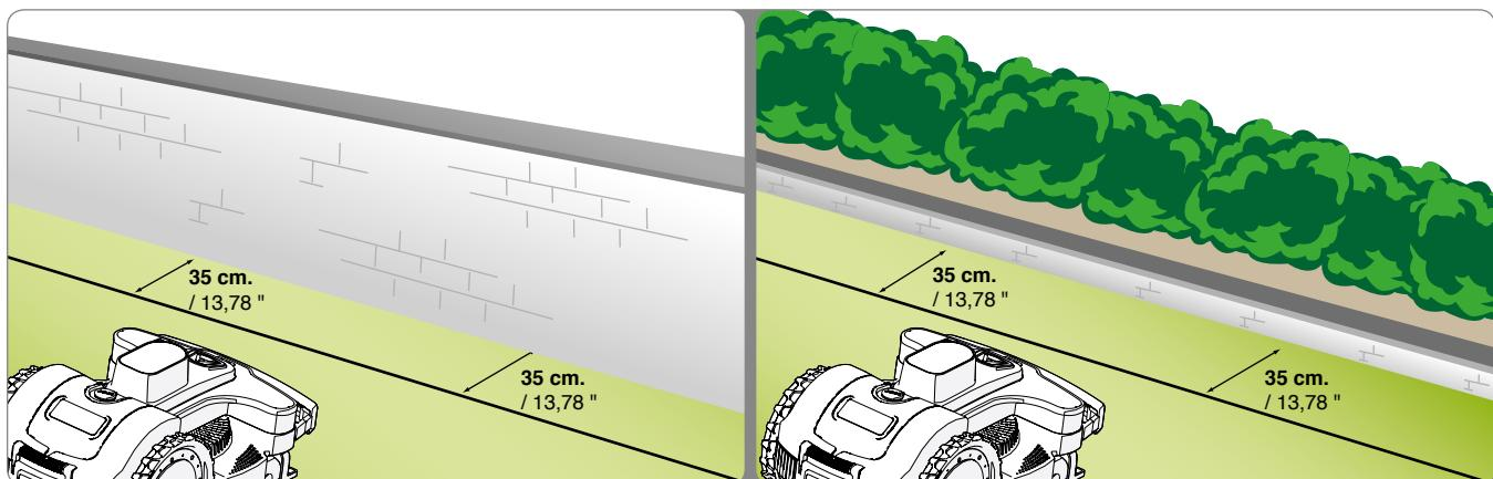
If a flower bed, hedge, plant with protruding roots, small ditch of 2-3 cm or small kerb of 2-3 cm is present inside or outside the work area, lay the perimeter wire at least 30 cm (11.81") from the obstacle to prevent damage being done to the robot or the obstacle.
