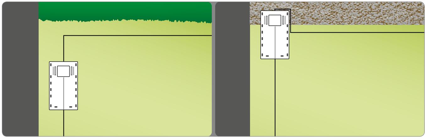
4. Fasten the charging station (N) to the ground with the pegs (P). If necessary, secure the charging station with screw anchors (Q).
