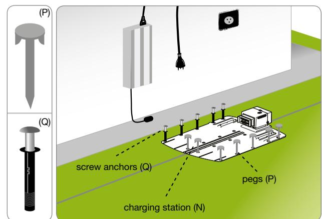
5. Install the power supply unit (A).
