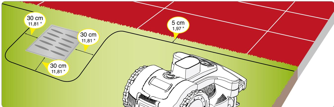
If an obstacle is present inside or outside the work area, such as a kerb or wall, lay the perimeter wire at least 35 cm (13.78") from the obstacle. Increase the distance between the perimeter wire and the obstacle; if you don't want the robot to hit the obstacle, place the perimeter wire at least 40 cm (15.75") away from it. Any grass close to the edge and outside the defined work area can be cut with a grass trimmer or brushcutter.
