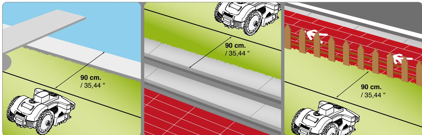
Obstacles resistant to knocks, such as trees, bushes or poles without sharp edges present inside the work area do not need to be delimited. The robot hits the obstacle and changes direction. If you don't want the robot to knock into the obstacles and for its safe and silent operation, all the fixed obstacles need to be delimited. Slightly sloping obstacles such as flower pots, stones or trees with protruding roots must be delimited to protect the cutting blade and the obstacles themselves.
